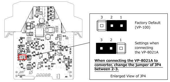
Fig.8-1 Jumper change when connecting the VP-8021A
