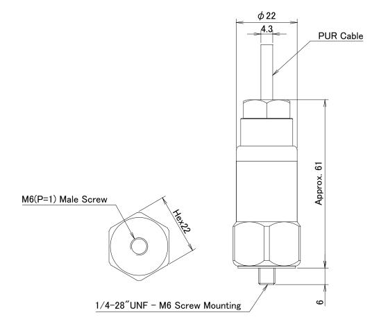
Outer Dimensions of the VP-1001000106 (Unit: mm)
