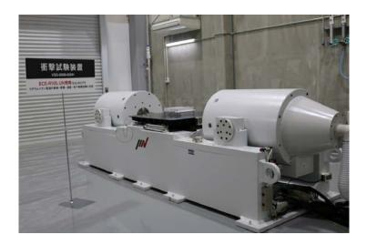
2) Vibration Testing Zone owns large sized test system which can respond to upsizing, long specimen up to 150kN, using push-pull method. To respond to user's various needs, also owns a horizontal vertical vibration test system (30-65kN) combined with a climatic chamber and a 3 axial earthquake resistance test system which can reproduce a real earthquake waveform.
